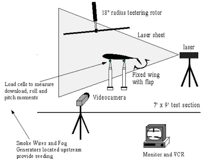
**Figure 3:** Schematic of experimental setup in Georgia Tech windtunnel.
