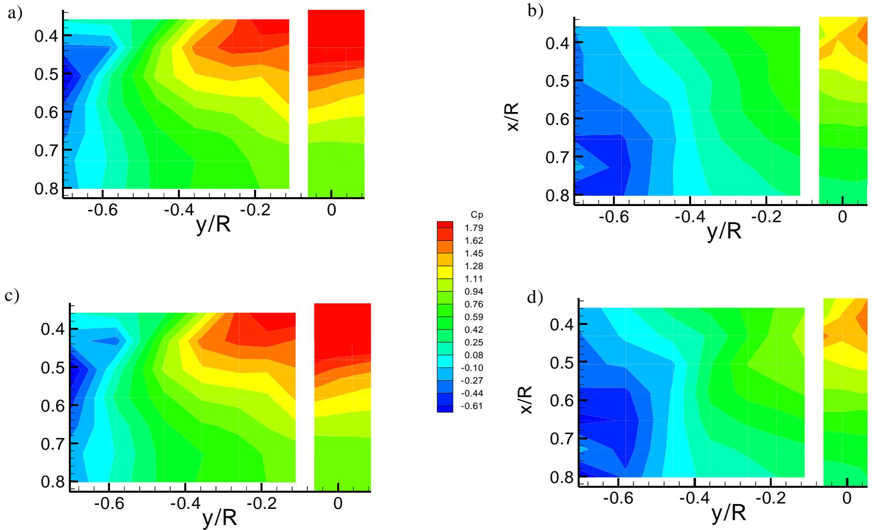
**Figure 4:** Static Pressure contours over the wing upper surface with segmented flap system at a)  $0^\circ$  b)  $30^\circ$  c) Outboard only flaps at  $30^\circ$  d) Inboard only flaps at  $30^\circ$
