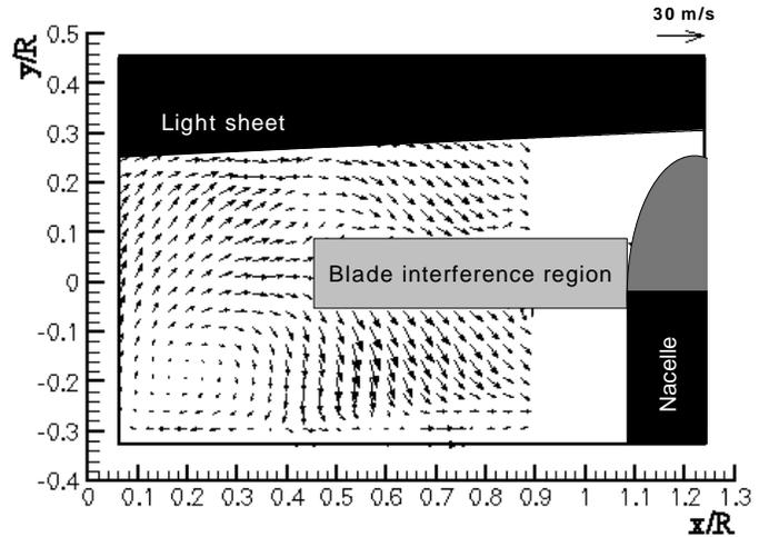
Figure 10: Time averaged velocity field for spanwise plane at 33% chord location
