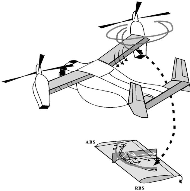
**Figure 1:** Correspondence of tiltrotor wing/rotor geometry during transition, to the geometry of the experimental configuration studied in the Georgia Tech John J. Harper 7' x 9' wind tunnel.
