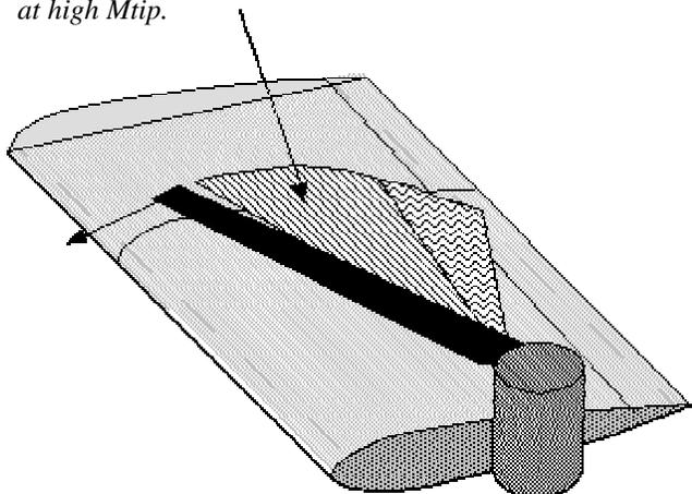
**Figure 12:** Schematic illustration of the phase lag between blade passage and pressure signature of the blade on the wing surface, when the rotor tip speed is in the compressible range.
