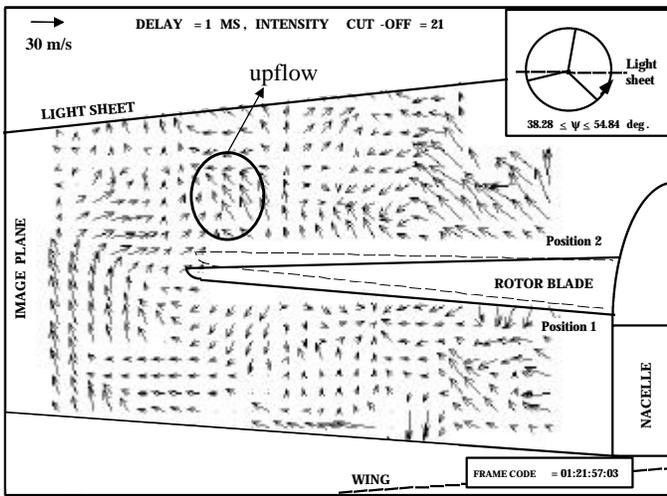
Figure 8: Spanwise Plane Instantaneous Velocity Field at 55% Chord Location
