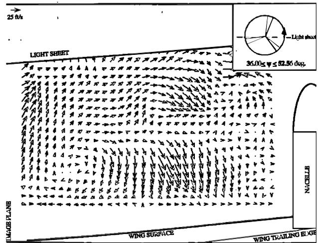
Figure 11: Ensembled-averaged velocity field at 55% spanwise plan for rotor azimuths between  $36^\circ$  and  $52.56^\circ$
