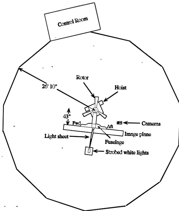
**Figure 6:** Typical measurement configuration for tiltrotor flows in a wind tunnel. Camera and light source distances to the measuring plane exceeded 5 meters. Facility borders are not to scale.
