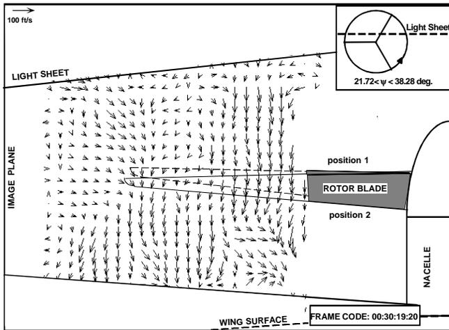
Figure 9: Spanwise Plane Instantaneous Velocity Field at 33% Chord Location
