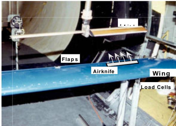
**Figure 2:** Photograph of experimental setup in Georgia Tech John J. Harper windtunnel
